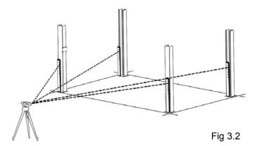
Note: The maximum shim thickness recommended by the factory is no more than 1/2" per Column using shims and anchors provided with the lift. A maximum shim thickness of 2" is possible by ordering optional shim plates. Contact your authorized BendPak Distributor for ordering information.
