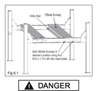
DO NOT PROCEED with Cable installation or go near the lift work area unless visual confirmation is made of ALL Safety Locks. ALL locks MUST be engaged before proceeding. Failure to comply with these instructions may result in severe personal injury or death. (See page 11)
