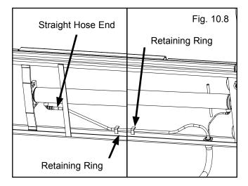
8. Connect the straight end of the Power Unit Hydraulic Line to the 90° Power Unit Fitting. Connect the Return Air Line to the 90° Air Fitting. There will be one air line hose left unconnected at this time. This air line hose will be used to activate the pneumatic safety locks on the next page. (See Fig. 10.9)
