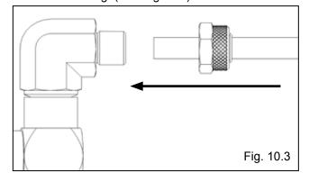
3. Install the 90-degree Hydraulic Fitting in the port at the ram end of the Cylinder. On the pipe thread side of the Fitting it is recommended to use Teflon Tape or pipe sealer. DO NOT USE TEFLON TAPE on the JIC flared end. (See Fig. 10.4)
