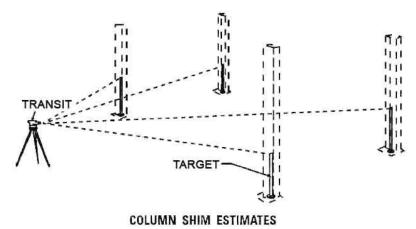
B. Place target on floor at column positions (NOT on column base plates) and record readings.
