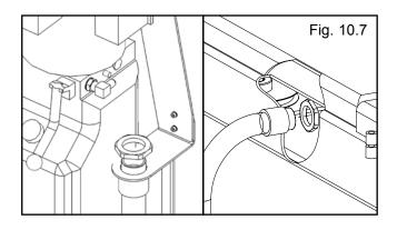
7. Connect the hydraulic hose and air line as shown below making sure the hydraulic hose passes through the retaining rings. MAKE SURE HOSES ARE KEPT CLEAR OF CABLES. There will be one air line hose left unconnected in this step. This air line will be used to activate the pneumatic safety locks in the next step. See pages 19 & 20 for Compression Fitting instructions. (See Fig. 10.8)
