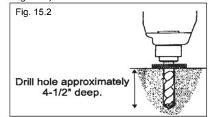
3. After drilling, remove dust thoroughly from each hole using compressed air and/or bristle brush. Make certain that the Columns remain aligned with the chalk line.
