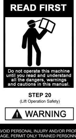
TO AVOID PERSONAL INJURY AND/OR PROPERTY DAMAGE, PERMIT ONLY TRAINED PERSONNEL TO OPERATE LIFT. AFTER REVIEWING THESE INSTRUCTIONS, PRACTICE USING LIFT CONTROLS BY RUNNING THE LIFT THROUGH A FEW UNLOADED CYCLES BEFORE LOADING VEHICLE ON LIFT. **NEVER** RAISE JUST ONE END, ONE CORNER, OR ONE SIDE OF VEHICLE.
