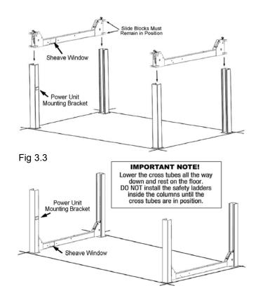
4. With the Columns standing and the crosstubes in position, install the Safety Ladders. Pass the Ladders through the Column openings and drop down through the Slide Block guide slots on the Crosstube until the Ladders come to rest on the Base Plates. If bolting, **DO NOT BOLT** Columns down at this time. (See Fig. 3.4 - 3.5)
