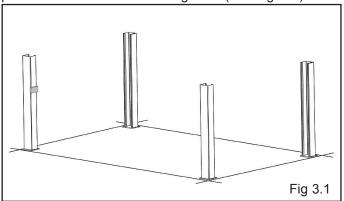
2. To estimate the shim requirements, place a target on floor at each Column position and record the readings. Find the highest of the four locations then find the difference between each of the remaining Columns. This difference is the estimated amount of shim thickness that will be required at each Column. (See Fig. 3.2)
