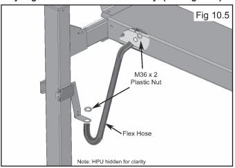
5. Connect Hoses as shown below making sure to pass through the retaining rings. Connect Power Hose (90° Fitting End) to Cylinder. MAKE SURE HOSES ARE KEPT CLEAR OF CABLES. (See Fig. 10.6)
