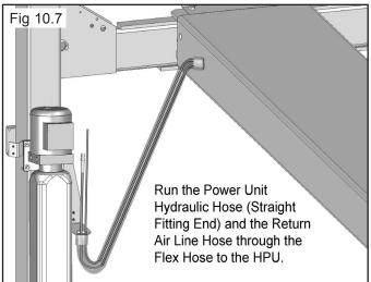
7. Connect the Power Unit Hydraulic Line (Straight Fitting End) to the 90° Power Unit Fitting. Connect the Return Air Line to the 90° Air Fitting. (See Fig. 10.8)
