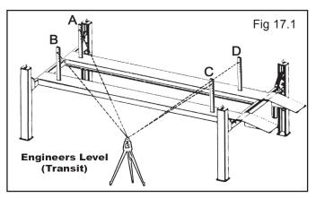
5. Beginning with "A" position, sight the level to the target and mark the number or the graduation on the inch scale of the target that aligns to the cross hairs of the Level. (See Fig. 17.1)
