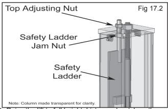
12. Raise the lift to full height. Listen and watch as the primary safeties engage the safety ladder. Synchronize by adjusting the cables so that all four latches click at same time. Make necessary adjustments to the cables allowing compensation for stretch.
