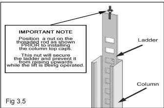
5. Install the Column TOP CAPS using the M16 x 2 nuts and M8 Hex Bolts, nuts & washers. Install the nut on each Safety Ladder until 1" of threads are exposed and the Ladder is raised at least 1/2" off of the base of the Column. NOTE: Raise the Ladder at least 1/2" off of the base of the column or damage to the lift will occur. Be sure to position the cable hole INWARD. (See Fig. 3.6 - 3.7)
