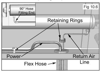
6. Run the Power Unit Hydraulic Hose (Straight Fitting End) and the Return Air line through the Flex Hose to the Power Unit. (See Fig. 10.7)
