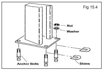
6. After any necessary shims are installed, tighten each nut 3-5 turns past hand tight. IMPORTANT - If anchor bolts do not hold when tightened to indicated amount, concrete must replaced. Saw cut and remove 24" x 24" square area each column base then re-pour with reinforced 2500 PSI concrete to a depth of six inches minimum, keying new concrete under existing floor. (See Fig. 15.5)
