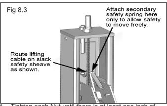
4. Tighten each Nut until there is at least one inch of threads protruding through the top of the nut. The Cables will remain loose until start up and final Cable adjustments are made. (See Fig. 8.4)
